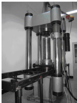
Fig.1 RLW-2000 岩石三轴流变试验机 Fig.1 Rock rheological test machine RLW-2000
