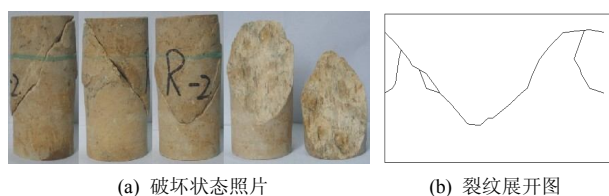
图10 R-2 破坏特征图 (方案 I, \sigma_3=30 MPa) Fig.10 Failure characteristics of sample R-2 (scheme I, \sigma_3=30 MPa)
