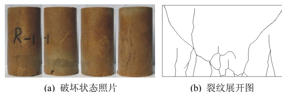
图12 R-1 破坏形态 (方案 II, \sigma_3=30 MPa) Fig.12 Failure characteristics of sample R-1 (scheme II, \sigma_3=30 MPa)
