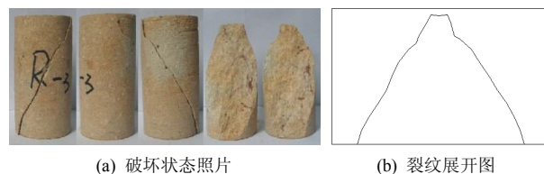
图9 R-3 破坏特征描图 (方案 I, \sigma_3=10 MPa) Fig.9 Failure characteristics of sample R-3 (scheme I, \sigma_3=10 MPa)
